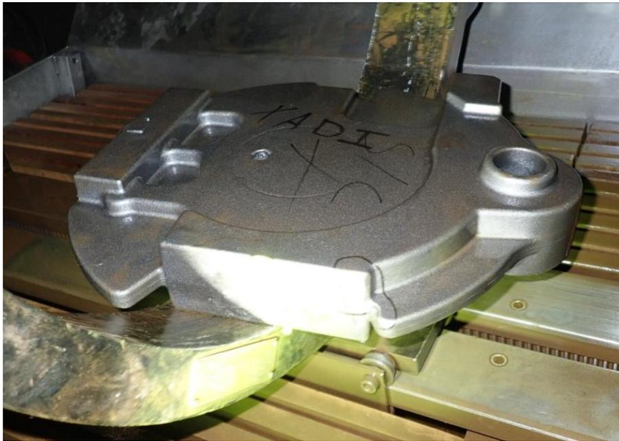
Figure 3-13. Indirect magnetization was performed at Foundry 3
