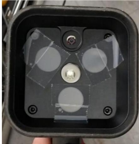
Figure 2-6. Camera with modified surrounding UV Lights
