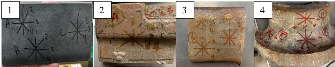
Figure 4-18. 1) Flat geometry with flush contact points, 2) Curved geometry with flush contact points 3) Flat geometry with irregular contact points, 4) Curved surface with irregular contact points
