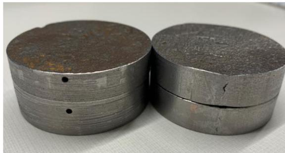
Figure 4-12. The puck-shaped samples containing sub-surface and surface defects.
