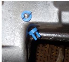
Figure 3-8. Magnets are used to mark the beginning and end of the crack.
