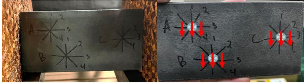
Figure 4-22. Left: Rectangular block setup on bench; Right: Orientation of magnetic field direction on the tested points of the rectangular block
