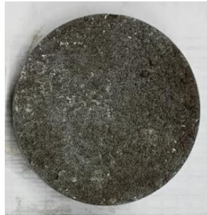
Figure 4-8. A puck-shaped sample machined from casting plate.
