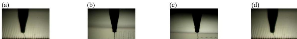
Figure 29. Representative images for different scenarios: (a) Normal printing (Scenario 1); (b) Change of filament dimensions (Scenario 2), (c) Tilted micro-filament (Scenario 3); (d) Multi-layer printing (Scenario 4)
