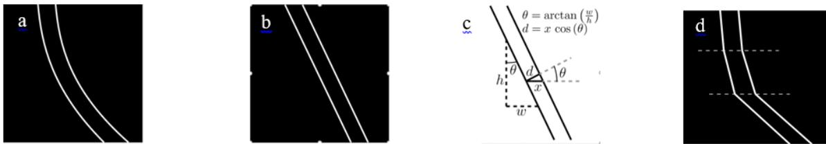
Figure 28. (a) A typical edge image of the tilted filament; (b) Approximate edge image; (c) Diameter and tilt-angle calculations; (d) Piecewise approximate edge image
