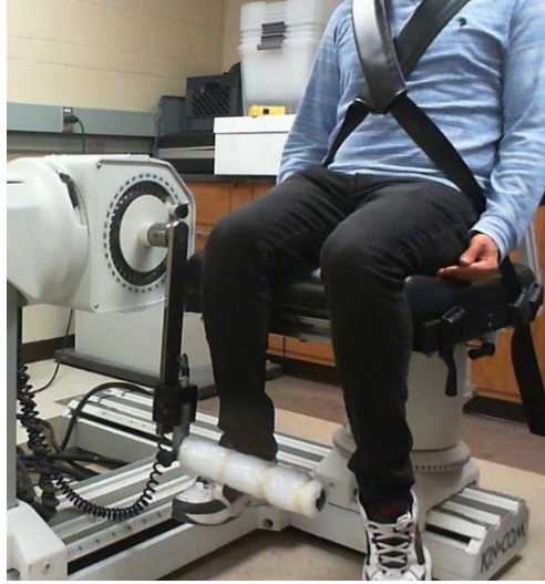
Figure 4.2 Apparatus and participant's position for rectus femoris exertions
