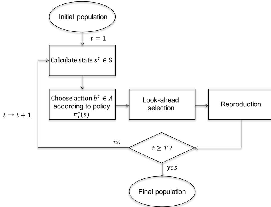
Figure 5.2 The simulation flowchart. The process starts with the initial population and goes through resource allocation, selection and reproduction steps until getting to the deadline. To find the optimal resources, we first calculate the current state and then take the action with highest value according to the optimal policy. The action represents the number of progeny to be produced for that generation.
