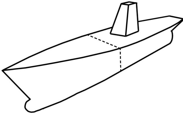
**Figure 1.** A model ship with a line where a new mid-section will be inserted.
