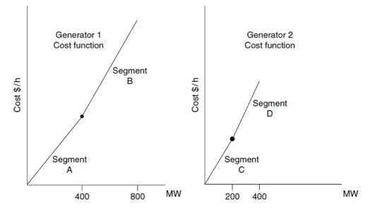
When performing economic dispatch, the calculation simply begins increasing the generation on the segment with the lowest marginal price (slope) until a limit is hit or the segment MW limit is hit. Therefore,
