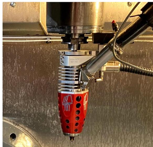
Figure 2. Extruder with 3mm nozzle
