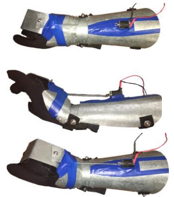
Figure 29: ARCTiC LawE Vrs. 2 (Top) Top down view - unactuated (Middle) Side view - actuated (Bottom) Top down view - actuated
