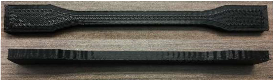
Fig 8(a): Specimen with 0.1mm layer thickness, 60mm/s printing speed &  $0^0$
