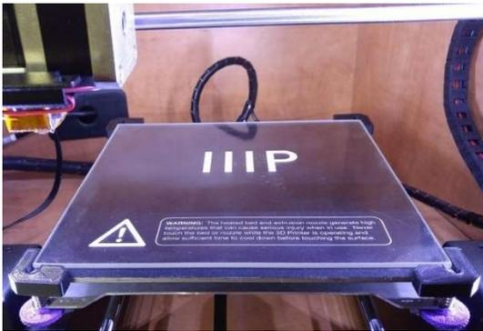
Fig 4: Build platform with a manual levelling mechanism
