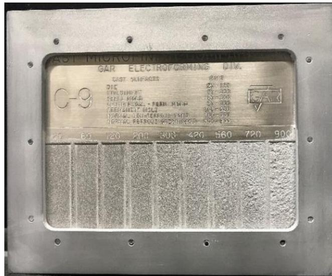
*Figure 24: Fixture used in study to bolt the three 'C-9' comparator plates*
