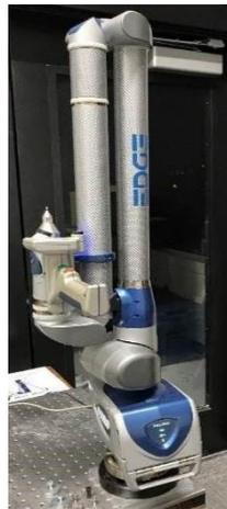
*Figure 12: Faroarm Edge with laser line probe.*
