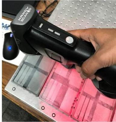
*Figure 42: HandyScan700 capturing point cloud of SCRATA plates*
