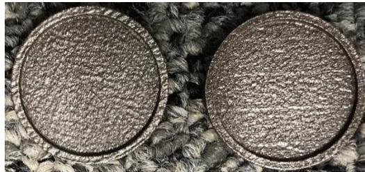
Figure 45: SS316L sample as fabricated by DMLS process
