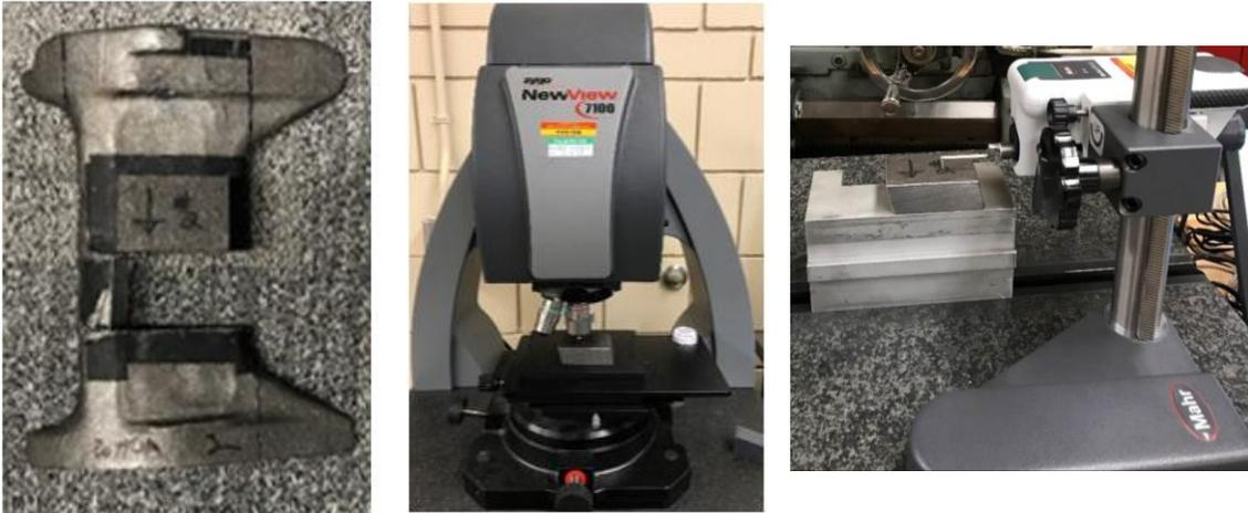
Figure 38 : Cut samples from Casting B and sample measurement using Zygo surface profiler and Mahr profilometer
