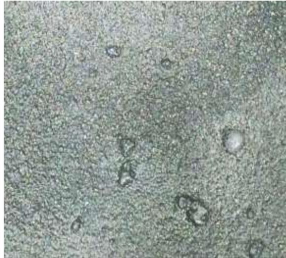
**Figure 1.1**—Porosity abnormalities on a casting
