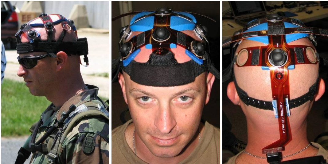
Figure1. The B-Alert EEG System adapted for use under a helmet in ambulatory conditions
