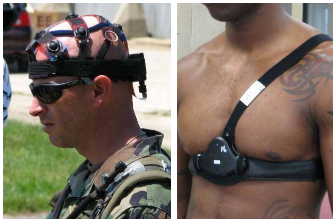
Figure 1. EEG (left) and ECG (right) sensors.
