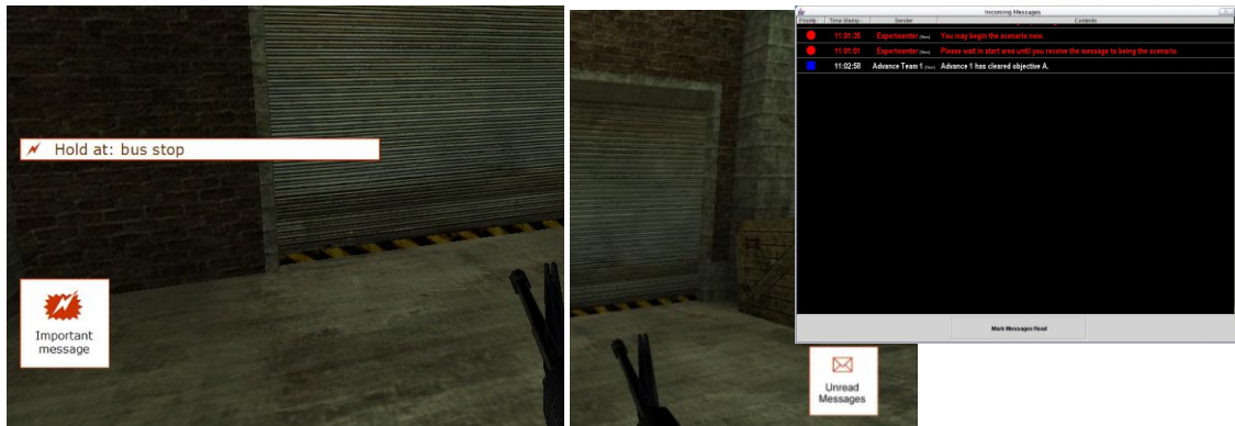
Figure 3. High priority messages are alerted by an icon and (possibly) a text summary on the HUD (right). Deferred messages appear on the Tablet PC with an icon on the HUD (left).
