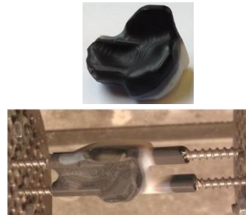
Figure 13. Implementation examples using designed sacrificial supports in the machining process.
