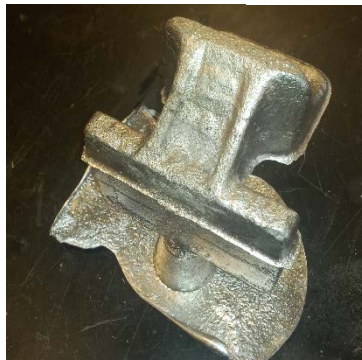
Figure 4.6(e). RECasted Aluminum Part
