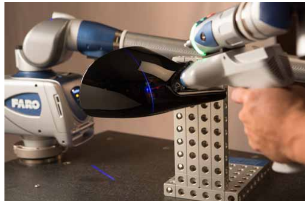
Figure 1.1. 3D Laser Scanner Working
