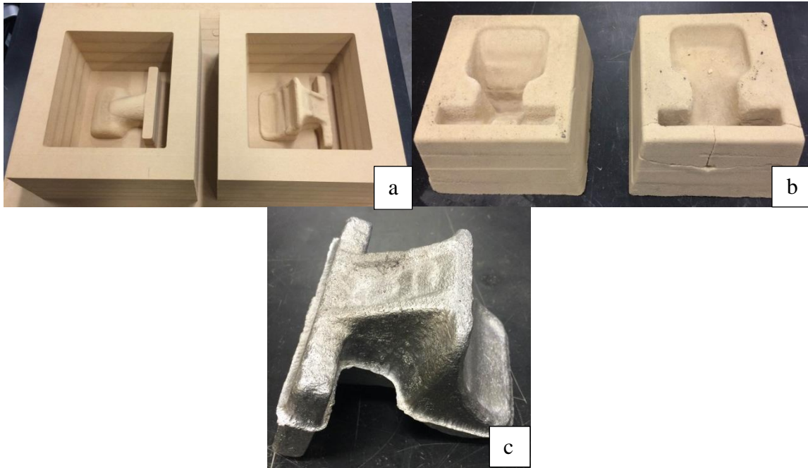
Figure 1.3: Samples from the RPM process, (a) wood patterns, (b) sand molds, and (c) resulting metal part
