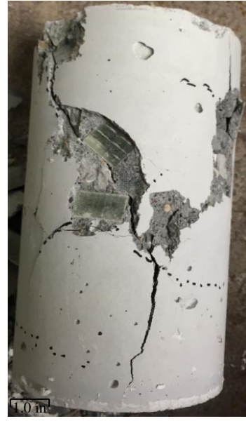
Figure 18: Compressive failure along cracking caused by curing
