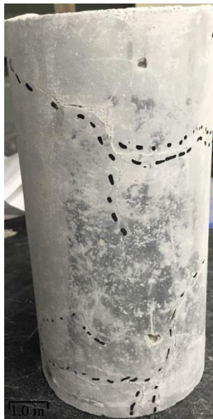
Figure 17: Cracking seen on samples stored in hot bath
