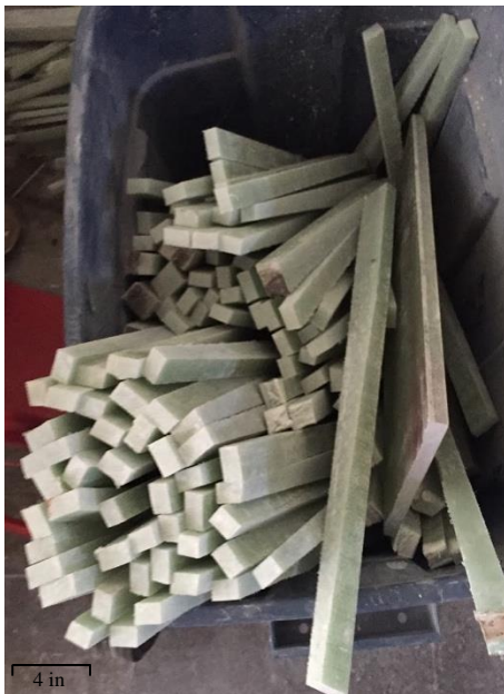
Figure 2: Strips of material cut by wet saw
