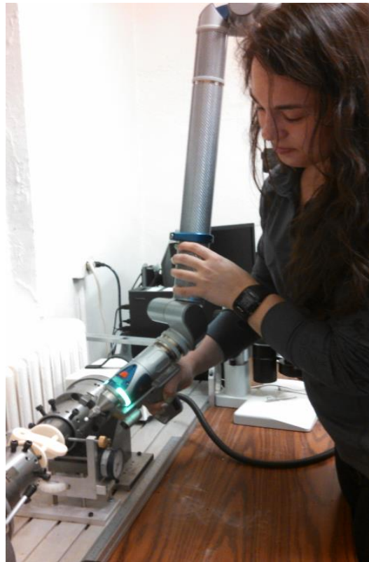
Figure 13. Coordinate metrology using Faro Arm
