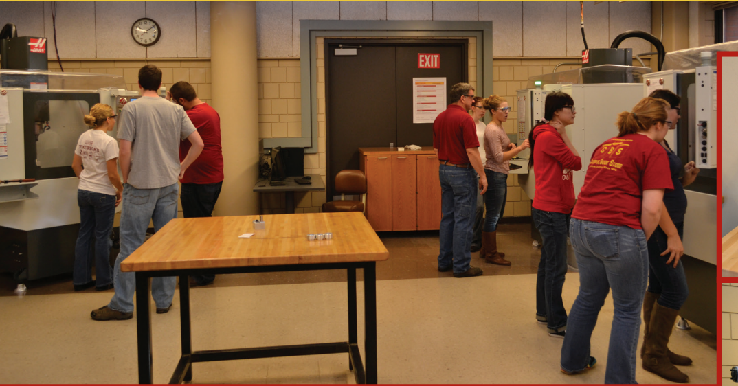
Four Haas CNC vertical milling machines are used to teach CNC programming and machining in several classes, including IE 248: Engineering System Design, Manufacturing Processes and Specifications, shown above. One of the machines is equipped with a Renishaw probing and tool setting system, and an optional 4th axis of control.
