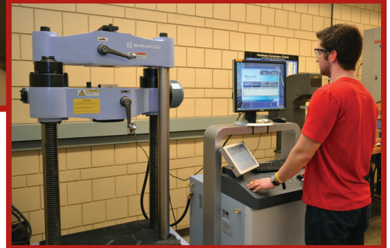
Above: New material testing & forming equipment includes (clockwise, from top) three Rockwell hardness testers, a laboratory rolling mill, and two Shimadzu tensile testing machines.
