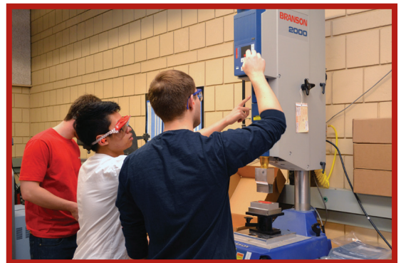
Above: Students in IE348: Solidification Processes work on the new Branson ultrasonic welder for polymer joining.
