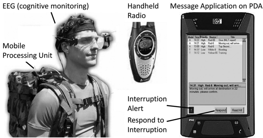
Figure 1. The Communications Scheduler includes an electroencephalogram-based cognitive monitoring system to assess workload, a handheld radio for aural messages, and a handheld PDA for text messages.
