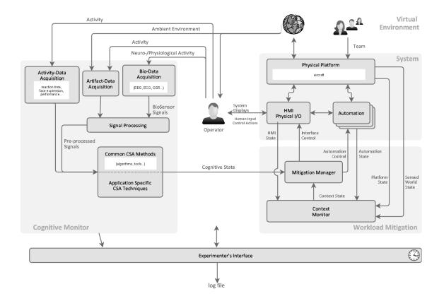
The system will consist of five main components: the cognitive monitor, the workload mitigation, the system, the virtual environment, and the human operator.
